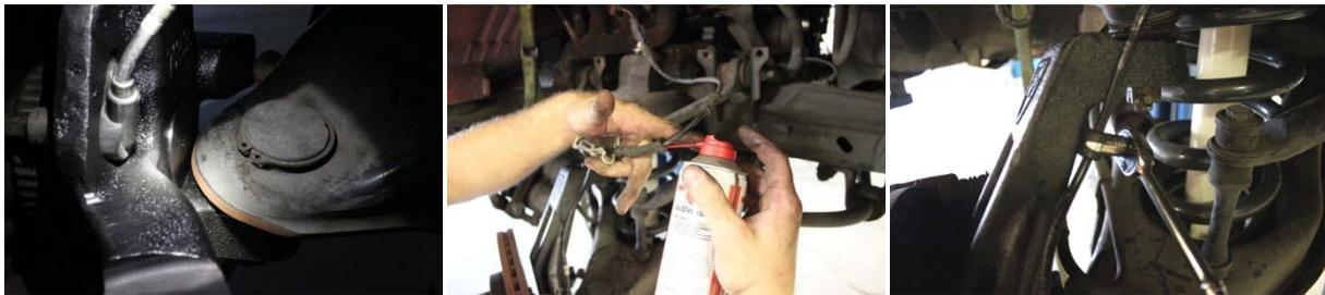
15. Reattach brake line guide to upper control arm and move the spindle throughout its turning cycle to ensure ABS line has plenty of slack.
