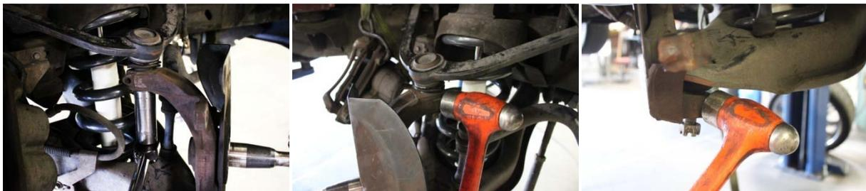
9. Install Maxtrac Suspension's lifted spindle, and tighten the upper and lower ball joints.
