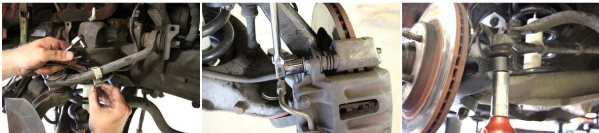
17. Depending on the year of the vehicle, you may have to grind down the front lip of the lower control arm about  $\frac{1}{4}$ ". Grind smooth, then paint to protect the raw metal of the arm.
