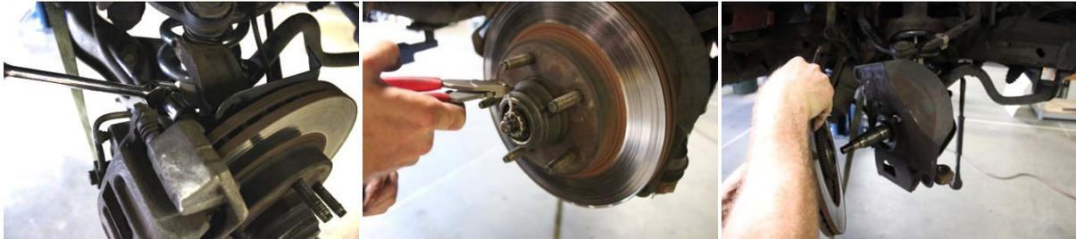
4. Unbolt and remove ABS sensor from spindle and the upper control arm.
