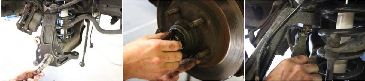
12. Install the ABS sensor into the new spindle, using the provided hardware.
