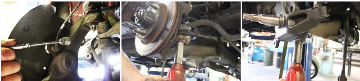
7. Loosen the upper ball joint nut, but do not remove. Break the upper ball joint loose from the spindle by smacking it with a hammer, make sure to hit the spindle, and not the threads/nut.
