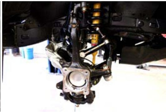
7. Remove the cotter pins from the tie rod and upper ball joint.
