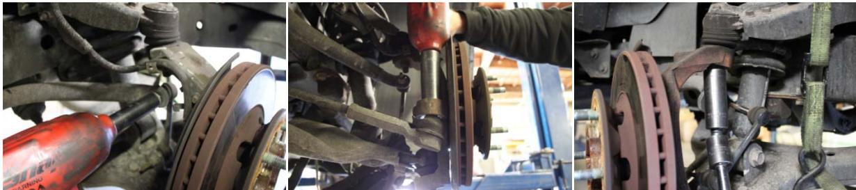
8. Loosen lower ball joint nut, but do not remove. Break the ball joint loose by hitting the side of the spindle with a hammer, then remove the nut and spindle.
