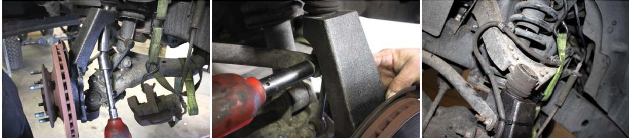
16. Remove the brake clip for the brake line at the frame to allow slack in order to bolt up the caliper. Provided are some gold washers that may need to be installed between the caliper and the spindle to ensure proper spacing of the rotor between the calipers mounting bracket.
