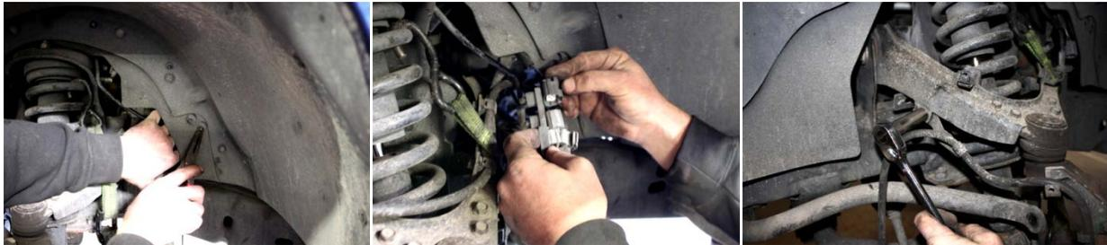
5. Unbolt sway bar end link at the sway bar and then separate.
