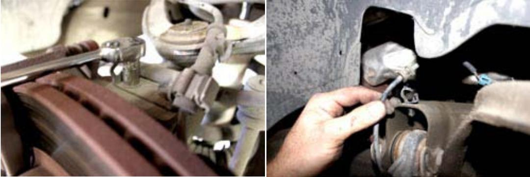
5. Remove the brake caliper (18mm socket), and then remove the brake rotor and set aside.
