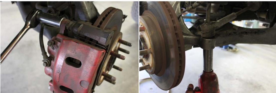
18. Below is the installation of the brake line bracket on the knuckle, also the suggested re-routing of the ABS line and brake line, both on one side of the knuckle, zip-tied together.
