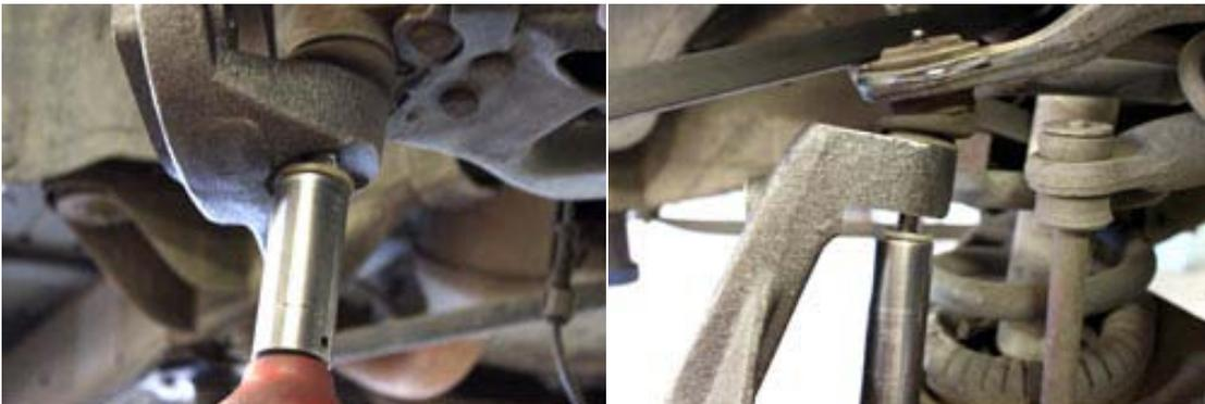
15. Make sure that the brake line has enough slack when moving the knuckle from full left turn to full right turn, make sure that the brake line is not pulled after the bracket is installed. It's also suggested to spray the brake line, at the knuckle bracket, with lubricant to make sure enough slack is present to install the brake line on the knuckle. Repositioning of the brake line bracket may be necessary, use stock hardware.
