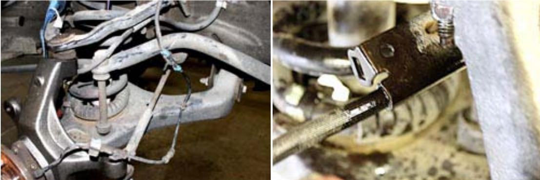
16. Reinstall the brake caliper and tighten with 18mm socket to factory specifications.
