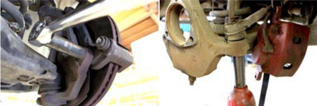
7. With the floor jack underneath the lower control arm, lift it up slightly to be able to remove the upper ball joint from the top of the knuckle (18mm).
