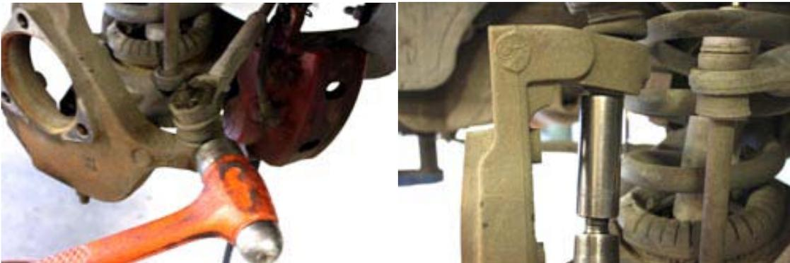
8. Remove the upper ball joint by striking it, or by using a ball joint separator.
