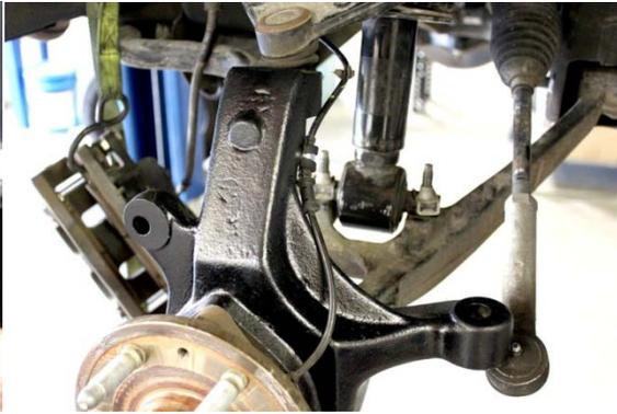
13. Install the extended brake lines using the provided clips, install the frame side first and allow fluid to run through the line before installing the caliper side. This will ease the bleeding process.
