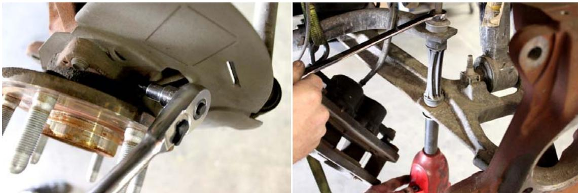
4. Unbolt unit bearing, remove and discard dust shield (will not be used). Unbolt tie rod from the spindle, then knock tie rod loose by hitting the side of the spindle, do not hit tie rod or threads!
