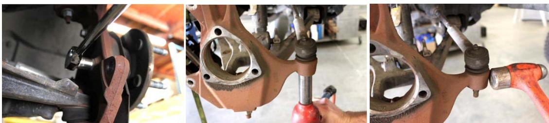
5. Loosen the upper ball joint nut, loosen the lower ball joint nut and leave the nut loose on the end of the threads, then knock the upper ball joint loose by striking the spindle (do not hit the threads!)
