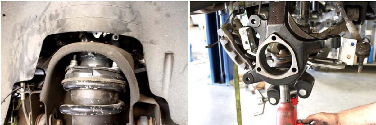
7. Tighten the upper ball joint nut, then tighten the lower ball joint nut.
