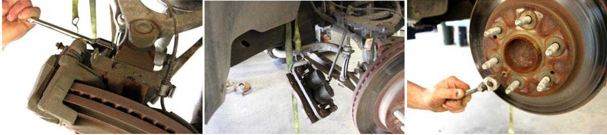
2. Open up brake hose clamp on upper control arm and remove from bracket. Unbolt brake hose bracket from upper control arm, then unbolt abs wire bracket from the spindle.
