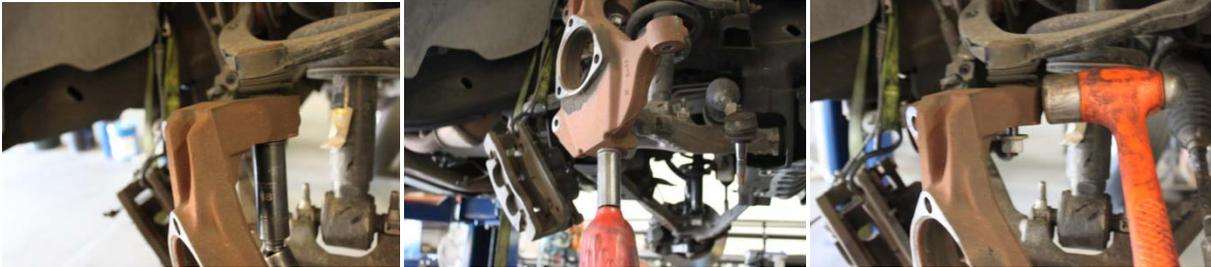
6. Support lower control arm and add pressure with a jack, then line up Maxtrac spindle with upper & lower ball joint, and loosely install nuts.
