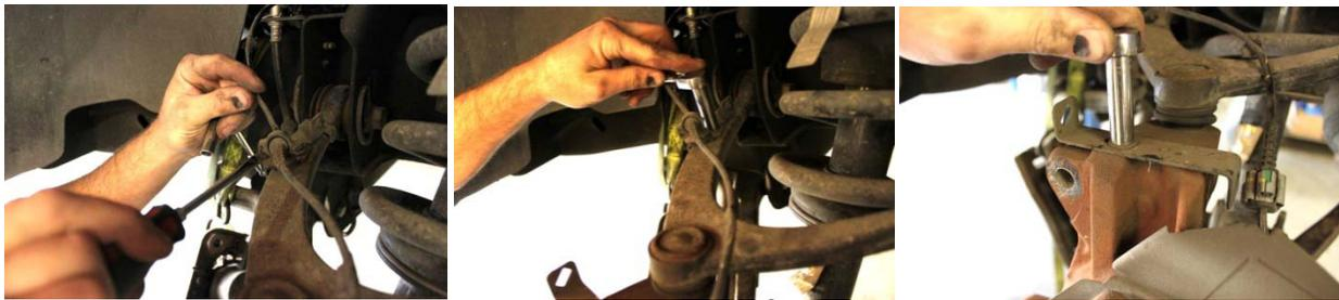
3. Remove ABS sensor from spindle and put it safely out of the way. Remove through bolt for sway bar end link and linkage.
