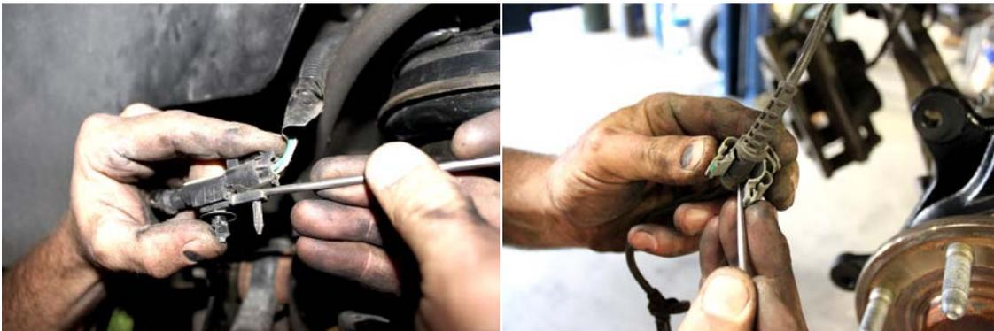
10. Use the provided Adel Clamp and factory bolt to attach ABS wire to upper control arm.
