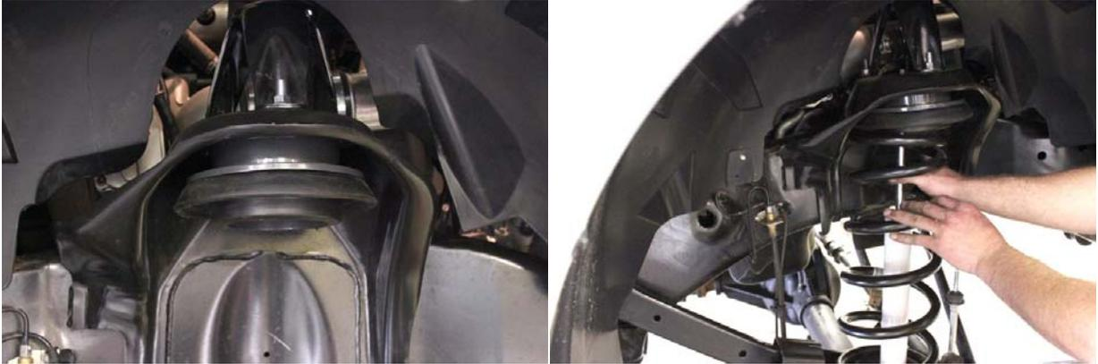
8. Install lower shock bolt and tighten to factory spec, repeat these steps on the other side of the vehicle.
