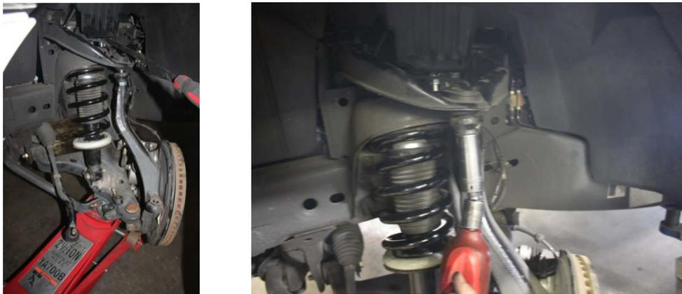
8. Repeat steps 1 through 7 on the passenger side of the vehicle, then re-install the sway bar nuts on both sides and re-torque to the factory specs.
