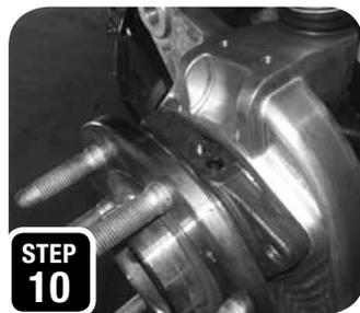
**STEP 10:** Re-install the wheel bearing using the factory bolts and 14mm provided washers.
