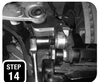
**STEP 15:** Attach the tie rod to the spindle and tighten
