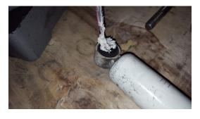
2) Lube up your shock bushings thoroughly with grease or lubricant.
