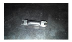
The bar pin should look like this when chamfer Is complete.
