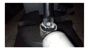
3) Press the bar pin into the bushing using a Press or vice. The chamfered end will funnel Itself into the bushing.
