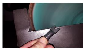
1) Use a sander or a grinder to chamfer one End of the bar pin
