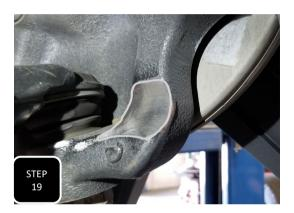
**Step 19** Using a 4.5" angle grinder with a flap disk or grind wheel, clearance this marked strike zone about 1/8" deep at the area of the contact point and smoothely transition your grind up and down.
