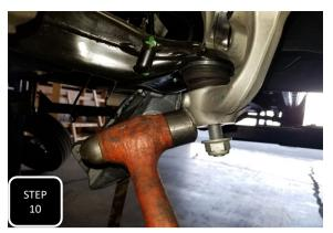
**Step 10** Loosen the nut attaching the lower ball joint to the spindle, but do not remove. Next, hit the side of the spindle, right at the ball joint, with a hammer, to break it loose and the nut will catch the spindle. Then remove the spindle. **NOTE: NEVER HIT THE BALL JOINT ON THE THREADS.**
