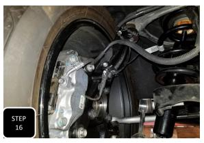
**Step 16** Attach the last guide bracket for the ABS and brake pad wires to the back side of the upper ball joint boss on the spindle using the factory M6 bolt and tighten.
