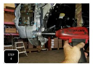
**Step 4** Unbolt both brake caliper mounting bolts and support the brake caliper up out of the way. **NOTE: NEVER ALLOW THE BRAKE CALIPER TO HANG BY THE BRAKE LINE.**
