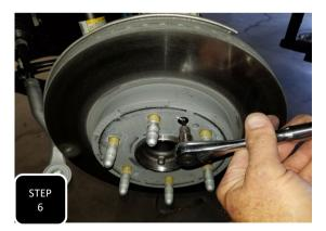
**Step 6** Unbolt the rotor retainer bolt and remove the rotor.
