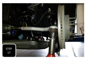
**Step 17** Lastly, attach the tie rod and tighten using the factory nut then repeat steps 1-17 on the other side.
