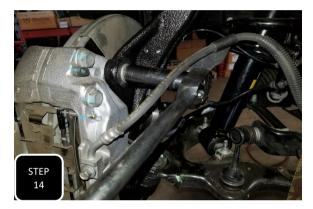
**Step 14** Attach the rotor by tightening the factory retainer bolt and then install the brake caliper using the factory bolts and tighten.
