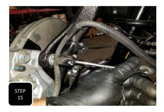
**Step 15** Attach the brake pad sensor wire to the neck of the spindle using the factory M6 bolt and then do the same with brake line bracket using the factory M6 bolt and tighten.
