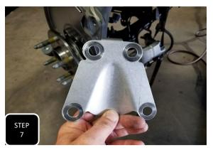
**Step 7** Remove the 4 bolts attaching the wheel bearing to the spindle and discard the 4 bolt plate between the bolts and the bearing.
