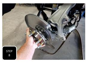
**Step 8** Separate the wheel bearing along with the dust sheild from the spindle and set aside for re-installation.
