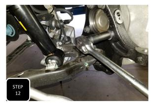
**Step 12** Install the wheel bearing along with the factory dust shield using the factory bolts and tighten.
