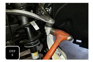
**Step 9** Loosen the nut attaching the upper ball joint to the spindle, but do not remove. Next, hit the side of the spindle, right at the ball joint, with a hammer, to break it loose and the nut will catch the spindle. **NOTE: NEVER HIT THE BALL JOINT ON THE THREADS.**
