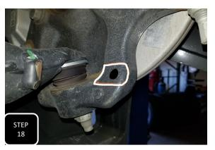
**Step 18** Start first by driving the truck and cycling the steering a few times to full turn so that a contact mark is left in the strike zone. Next, put the truck up in the air and mark about a 1.5" vertical area around the impact mark. This will be the area to clearance.
