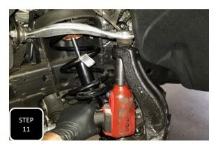
Step 11 Install the new spindle using the factory upper and lower ball joint nuts and tighten.
