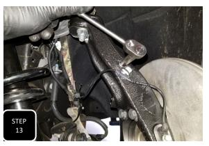
Step 13 Attach the ABS sensor and the wire guide just above it to the new spindle using the factory M6 bolts.
