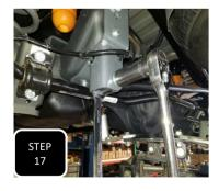
**Step 17** Attach the trac bar to the new bracket using the provided M14 bolt, nut, and washers. **NOTE: DO NOT FULLY TIGHTEN THE BOLT UNTIL THE TRUCK IS ON THE**
