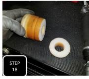
**Step 18** Remove the factory bump stops by popping them out of their mounting cup. Using a suitable cutting device, cut off half of the 1st rib of the bump stops and then reinstall them.
