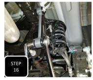
**Step 15** Install both shocks using the provided hardware at the top and the factory bolts at the bottom and tighten. **NOTE: DO NOT OVER TIGHTEN THE UPPER STEM BUSHINGS.**
