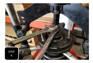
**Step 4** Using an automotive coil/strut compressor, compress the coil so that the strut can be disassembled safely and then remove the nut at the center of the strut top.
