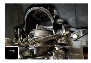
**Step 3** Unbolt the two mounting bolts at the bottom of the strut along with the three nuts at the top of the strut and remove the strut through the opening in the lower control arm.
