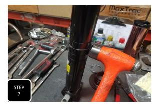
**Step 7** Slide the snap ring retainer over the snap ring. If the retainer does not slide over the ring, then tap the ring with a hammer to fully seat it and then install the retainer. **NOTE: THE RETAINER MUST GO COMPLETELY OVER THE SNAP RING AND SEAT OR YOUR SUSPENSION COULD FAIL.**
