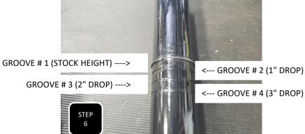
**Step 6** Locate your new struts and set the ring to the proper groove according to the chart above. Make sure the snap ring fully engages into the groove.
