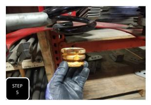
**Step 5** Once the nut is removed, remove the strut out from the bottom of the coil and then remove the bump stop.
