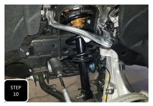
**Step 10** Re-install the strut top and tighten down using the provided M14 nylock nut. **NOTE: MAKE SURE TO PROPERLY CLOCK THE STRUT TOP WITH THE BOTTOM OF THE STRUT.**
