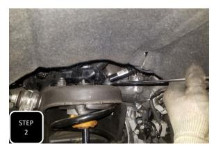
Step 2 3 Unbolt the two mounting bolts at the bottom of the strut along with the three nuts at the top of the strut.
