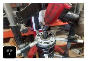
**Step 4** Using an automotive coil/strut compressor, compress the coil so that the strut can be disassembled safely and then remove the nut at the center of the strut top. **NOTE: TAKE NOTE OF THE RELATIONSHIP BETWEEN THE STRUT TOP AND THE STRUT BOTTOM FOR PROPER CLOCKING DURING INSTALLATION.**
