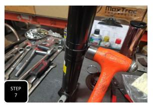
**Step 7** Slide the snap ring retainer over the snap ring. If the retainer does not slide over the ring, then tap the ring with a hammer to fully seat it and then install the retainer. **NOTE: THE RETAINER MUST GO COMPLETELY OVER THE SNAP RING AND SEAT OR YOUR SUSPENSION COULD FAIL.**
