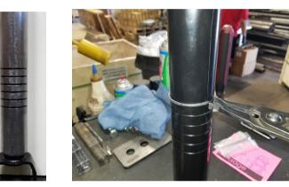
**Step 8** The new strut has 8 grooves for the specified year range and desired ride height. Choose your groove based on the chart above or the picture on the back of the instructions.
