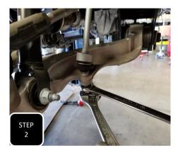
**Step 2** Un-bolt the sway bar end link at the lower control arm.
