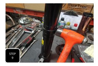
**Step 9** Slide the snap ring retainer over the snap ring. If the retainer does not slide over the ring, then tap the ring with a hammer to fully seat it and then install the retainer. **NOTE: THE RETAINER MUST GO COMPLETELY OVER THE SNAP RING AND FULLY SEAT OR YOUR SUSPENSION COULD FAIL.**
