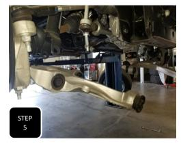
**Step 5** Remove the bolt attaching the strut to the lower control arm and allow the lower control arm to hang by the ball joint.
