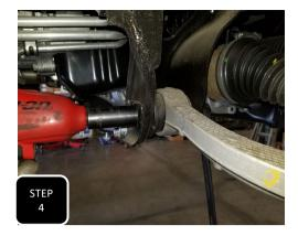
**Step 4** Un-bolt and remove both alignment cam bolts attaching the lower control arm to the frame.
