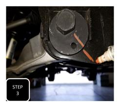
**Step 3** Make a reference mark on both alignment cam bolts as a guide when re-installing.
