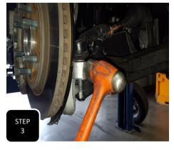
**Step 3 3** Unbolt the tie rod from the spindle. You may need to hit the side of the steering arm with a hammer to separate. **NOTE: NEVER HIT THE TIE ROD ON THE THREADS.**
