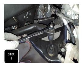
**Step 2** Unbolt the sway bar end link from the sway bar and separate.
