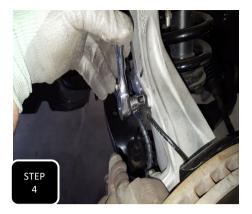
**Step 4** Unbolt the brake line guide and ABS line guide from the neck of the spindle and separate.
