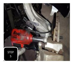
**Step 5** Unbolt the brake caliper and support out of the way, then remove the brake rotor.
