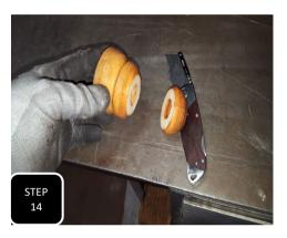
**Step 14** Install the supplied lower coil seat then cut down the factory bump stop by one rib and slide the bump stop onto the shock shaft.
