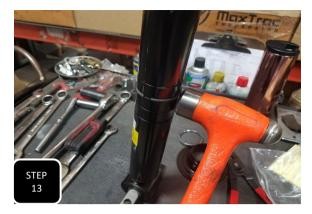
**Step 13** Install the snap ring retainer over the clip. If it does not slide over the clip, use a hammer to tap the clip into the groove until it fully seats. **NOTE: THE RETAINER MUST GO COMPLETELY OVER THE SNAP RING AND SEAT OR YOUR SUSPENSION COULD FAIL.**
