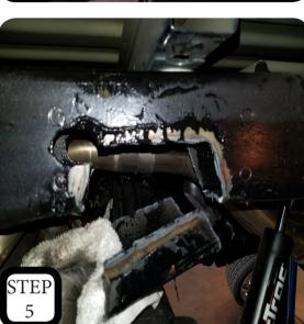
STEP 6: Test fit the frame support. If it fits all the way up and flush with the bottom of the frame, then clean up all the cut edges. If it does not fit flush, continue trimming until it does fit flush, then grind edges smooth.
