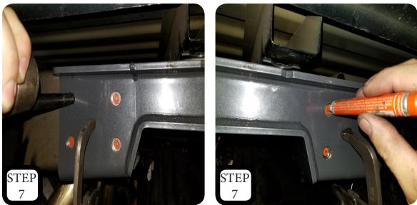
**STEP 7:** Clamp the frame support up into place on the frame and mark all the holes that need to be drilled. Next, center punch each hole using a transfer punch.
