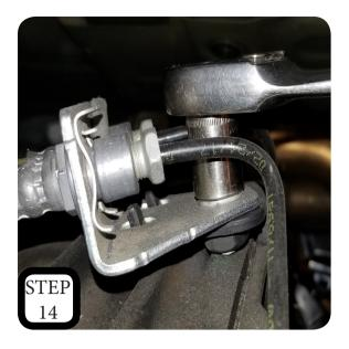
**STEP 14:** Unbolt the brake line bracket on top of the differencial.
