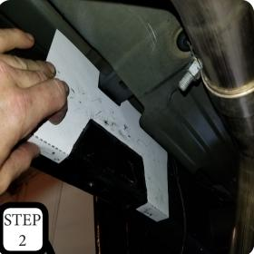
**STEP 2:** Cut out the supplied template, bend it on the dotted lines and line up with the frame and the bed rib.
