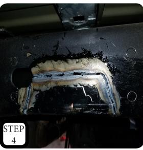
**STEP 4:** Using a plasma cutter, torch, or suitable cutting device; cut out the line that was scratched onto the frame.
