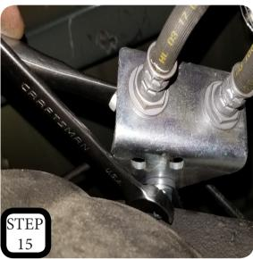
**STEP 15:** Pull the brake line bracket forward and loosely attach the provided brake line relocation bracket using the factory bolt at the diff and the provided 8MM bolt at the bracket. When all is lined up, tighten down both bolts.
