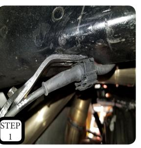
**STEP 1:** Unclip the ABS plug and line guides at the frame and move the line out of the way.
