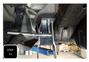
**Step 11** Locate the driver's side hanger and loosely install it into the driver's side, front leaf spring mount. Use the factory bolt at the main leaf spring hole and the provided 7/16" bolt, nut, and washer up through the top of the hanger. Tighten the 7/16" bolt first and then the main leaf spring bolt.
