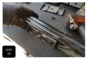
**Step 10** Slide the center pin through the factory 2 degree shim and install the pin down through the top of the leaf spring with the thick end of the shim facing the front of the truck. Then tighten the center pin. **NOTE: THE U-BOLT RETAINER PLATE DOES NOT GET RE-USED.**
