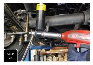
**Step 28** Install the new shorter shocks with the shaft of the shock attached at the frame and the body of the shock attached at the axle. **NOTE: IF YOU PURCHASED SHOCK EXTENDERS, NOW WOULD BE THE TIME TO INSTALL THEM ALONG WITH THE FACTORY SHOCKS. USE THE EXTENDER INSTRUCTIONS FOR INSTALL.**
