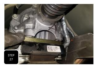
**Step 27** Remove both mounting bolts that attach the transmission to the mount at the cross member at the rear of the trans. Jack the trans up, insert the provided 1/2" tall, gold spacer, and tighten down using the factory bolts. **NOTE: THE USE OF THE PROVIDED 1/4"**, **SILVER SPACER MAY ONLY BE NEEDED IF DRIVE LINE VIBRATION IS EXPERIENCED.**
