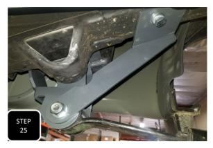
**Step 25** Install the hanger support bracket on the passenger side. The nut plate will get inserted through a hole on the inside of the frame this time and the rest will attach just like on the driver's side. Again, do not fully tighten the leaf spring bolt until the truck is on the ground at ride height.
