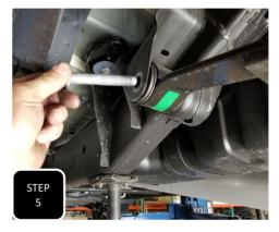
**Step 5** Loosen then remove the bolt attaching the spring to the frame at the front of the leaf spring and then remove the leaf spring.
