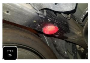
**Step 26** Insert the bump stop nut plates into the hole in the bottom of the frame that emerged after you removed the driver's and passenger's side factory bump stop plate. Thread the provided low profile bump stop into the nut plate until tight.
