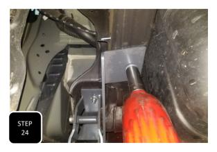
**Step 24** Loosely attach driver's side hanger support bracket using the provided M16 nut and washer at the hanger and the provided 1/2" bolt and washers at the frame. Tighten the 1/2" bolt at the frame, but do not fully tighten the 16mm spring bolt until the truck is on the ground at ride height.
