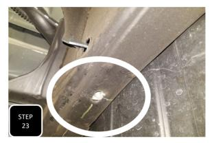
**Step 23** Insert the driver's side, zinc plated nut plate into the hole in the outside of the frame, just back from the front leaf spring mount. **NOTE: THE NUT WILL LINE UP WITH THE SLOTTED HOLE IN THE BOTTOM OF THE FRAME.**
