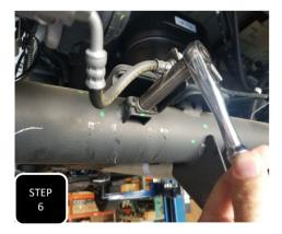
**Step 6** Unbolt the brake line guide bracket from the mounting bracket just under the spring perch on the axle and pull the line clear of the area.
