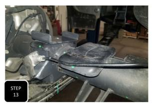
**Step 13** Place the axle relocator on top of the leaf spring with the brake line mounting bracket facing rearward and lower the axle into the relocator. **NOTE: IT WILL HELP THE LINE UP PROCESS TO LOOSEN THE U-BOLTS ON THE OTHER SIDE, BUT DO NOT REMOVE THEM.**
