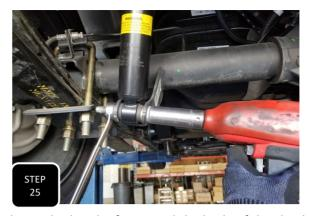
**Step 25** Install the new shorter shocks with the shaft of the shock attached at the frame and the body of the shock attached at the axle. **NOTE: IF YOU PURCHASED SHOCK EXTENDERS, NOW WOULD BE THE TIME TO INSTALL THEM ALONG WITH THE FACTORY SHOCKS. USE THE EXTENDER INSTRUCTIONS FOR INSTALL.**
