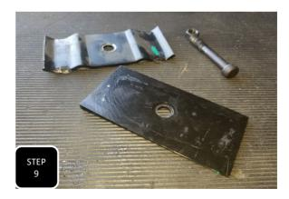
**Step 9** The leaf pack will now need to be dis-assembled. Attach two clamps to the spring and remove the center pin along with the U-bolt retainer plate and the factory 2 degree shim. **NOTE: DISCARD THE U-BOLT RETAINER PLATE. IT DOES NOT GET RE-USED.**
