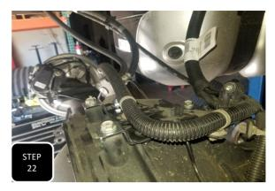
**Step 22** Locate the three "Z" shaped brake line brackets and loosely attach them to the factory bracket first using the provided hardware, and then to the diff using the factory hardware. The provided brackets are designed to push the factory bracket down and forward for more clearance between the diff and the bed.
