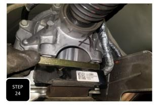
**Step 24** Remove both mounting bolts that attach the transmission to the mount at the cross member at the rear of the trans. Jack the trans up, insert the provided 1/2" tall, gold spacer, and tighten down using the factory bolts. **NOTE: THE USE OF THE PROVIDED 1/4"**, **SILVER SPACER MAY ONLY BE NEEDED IF DRIVE LINE VIBRATION IS EXPERIENCED.**
