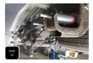
**Step 12** Jack up the axle and loosely re-install the leaf spring underneath the axle using the provided 16mm bolt at the front of the spring and the factory bolt at the shackle.
