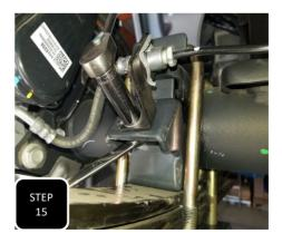
**Step 15** Locate the brake line mounting bracket still attached to the brake line and bend the guide tab to a flat position. Next, attach this bracket to the mounting bracket on the back side of the axle relocator using the provided M8 bolt, nut, and washer.
