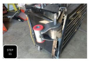
**Step 11** While the spring is out of the truck, install the new shackle using the provided 14mm bolt. Make sure to install the bolt in the same direction as stock, pointing away from the frame, and leave loose. **NOTE: DO NOT INSTALL A WASHER ON THE HEAD SIDE OF THE BOLT.**
