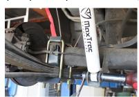
**10)** Do not tighten the leaf spring or shackle bolts until the vehicle is on the ground at ride height.
