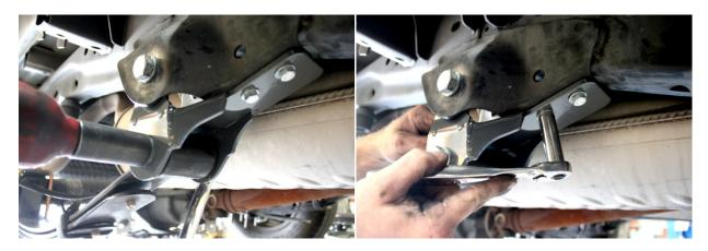
Have your truck re-aligned as soon as possible. Re-tighten all fasteners after 100 miles, then 500 miles.
