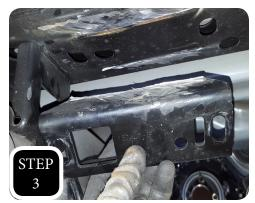
STEP 3: Cut the carrier bracket out at the welded bead. Once its seperated clean the area up with a grinder and spray paint for rust prevention
