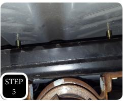
STEP 5: Jack up the driveshaft and align the holes, install using the provided M10-1.5 x 60MM bolts and hardware.
