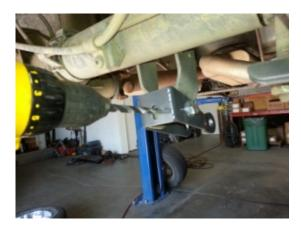
INSTALL THE PROVIDED 3/8" BOLT THROUGH THE DRILLED HOLE AND TIGHTEN ALL BOLTS. THEN INSTALL THE SHOCK IN TO THE ANGLE CORRECTOR USING THE ORIGINAL HARDWARE. (PIC 400900 INSTALLED)
