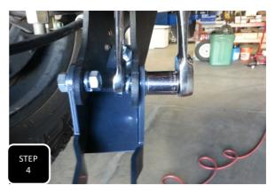
**Step 4** Tighten up the 7/16" bolt first and then the two 1/2" bolts.
