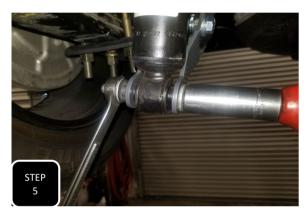
**Step 5** Attach the shock to the extender using the factory hardware and tighten.
