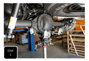
**Step 1** Jack up the rear of the truck and support under the frame rails with jack stands. Keep an adjustable jack under the axle for height adjustment.
