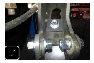
**Step 3** Slide the extender over the factory shock mount on the axle and loosely install the hardware. Install the flat washers onto the 1/2" bolts, install the 1/2" bolts through the factory shock hole, from the outside facing inward, then attach the 1/2" lock washer and jam nut. Then place the square plate over the ovalized opening inside the factory shock mount and attach it to the extender using the supplied 7/16" hardware.
