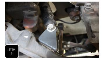
**Step 3** Attach the new shock mount using the factory hardware. Make sure the straight edge isfacing the engine. Next, attach the shock using the factory hardware and tighten. **NOTE: THIS EXTENDER IS INTENDED TO BE USED WITH A STOCK LENGTH SHOCK.**
