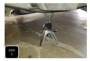
**Step 1** Jack up the front of the truck and support under the frame rails with jack stands.
