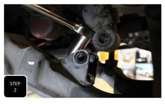
**Step 2** One side at a time, unbolt the shock from the mount on the control arm and then unbolt the mount from the control arm and remove.
