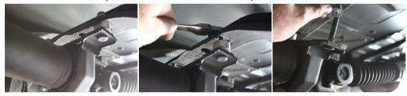
2) HOOK A TAPE MEASURE ON THE ORIGINAL CARRIER BEARING SLOTTED HOLE AND DRAW A LINE 3"OUTWARD: REPEAT ON OTHER SIDE.
