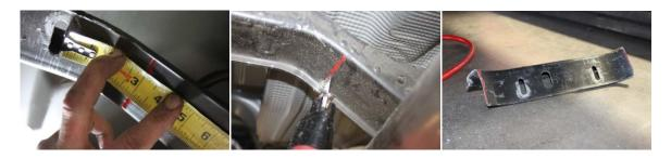
3) CUT THE CROSS MEMBER AT BOTH LINES AND REMOVE CENTER SECTION.
