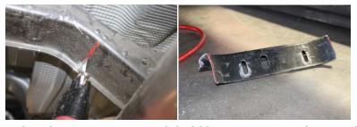
4) PUSH YOUR NEW MAX TRAC CROSS MEMBER UP TIGHTLY AGAINST THE ORIGINAL CROSS MEMBER AND CLAMP IT. ALSO INSTALL THE BOLTS ON THE VERTICAL SIDE OF THE CROSS MEMBER TO HELP HOLD IT IN PLACE.
