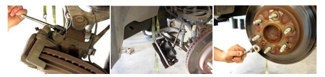
2. Open up brake hose clamp on upper control arm and remove from bracket. Unbolt brake hose bracket from upper control arm, then unbolt abs wire bracket from the spindle.
