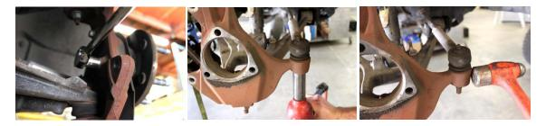
5. Loosen the upper ball joint nut, loosen the lower ball joint nut and leave the nut loose on the end of the threads, then knock the upper ball joint loose by striking the spindle (do not hit the threads!)
