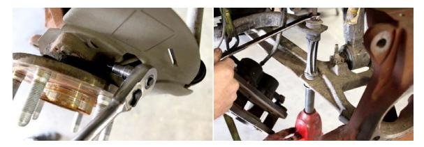
4. Unbolt unit bearing, remove and discard dust shield (will not be used). Unbolt tie rod from the spindle, then knock tie rod loose by hitting the side of the spindle, do not hit tie rod or threads!
