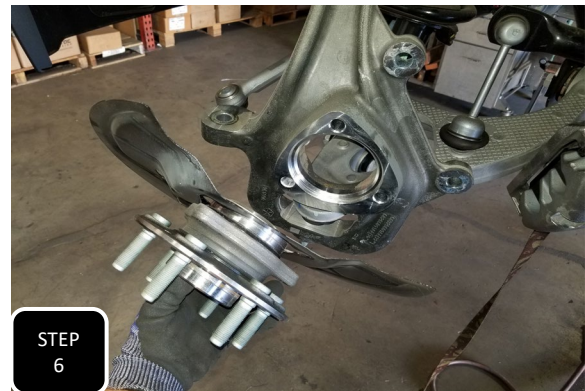
Step 6 Unbolt the 3 bolts attaching the wheel bearing to the spindle and remove the wheel bearing along with the dust shield.
