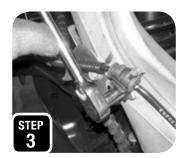
**STEP 3:** Unbolt the ABS wire guide bracket from the spindle, remove the plastic clamp and discard.
