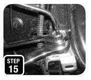
**NOTE:** 2015 MODELS WILL USE THE BRAKE LINE WITH THE THREADED ADAPTOR. 2009-2014 MODELS WILL NOT USE THE THREADED ADAPTOR.
