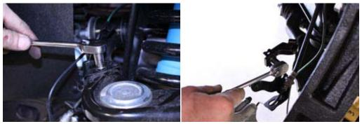
17. Bend the tab on the brake line bracket, then attach brake line bracket to the new spindle using the supplied hardware.
