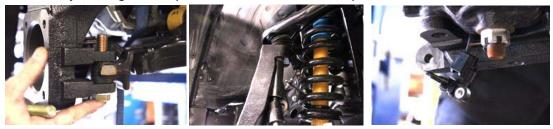
12. Attach lower ball joint / steering stop plate to the new spindle, tighten supplied 5/8"x3 ¼" bolts
