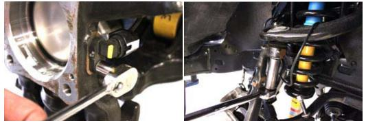
10. Remove bolts from lower ball joint / steering stop plate, then break upper ball joint loose by hitting the side of the spindle, do not hit the thread, remove stock spindle.
