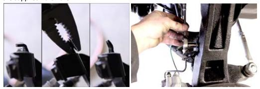
18. Remove stock brake line at the frame & caliper, then install new one. We suggest installing on frame side first, to let fluid bleed through the new line, then attach on caliper side.
