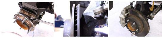
**NOTE:**If you are installing these spindles on a 2016+ 4runner, use the provided custom M12-1.25 x 40 bolts and 14MM washers to mount the brake calipers.
