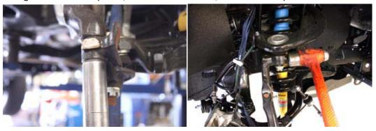
11. Guide ABS line down between the new spindle and lower ball joint/ steering stop plate. Slide lower ball joint into the double sheer mount & attach upper ball joint to new spindle, tightening nut on ball joint, align cotter pin hole & install OEM cotter pin.
