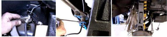
19. Tighten the new brake lines, per reversing the above steps.
