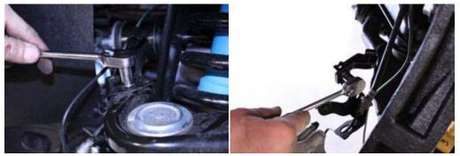
17. Bend the tab on the brake line bracket, then attach brake line bracket to the new spindle using the supplied hardware.
