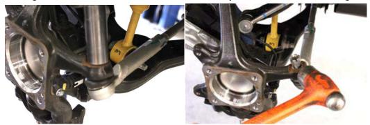
9. Remove the ABS Sensor, then upper ball joint nut.
