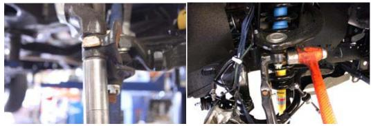
11. Guide ABS line down between the new spindle and lower ball joint/ steering stop plate. Slide lower ball joint into the double sheer mount & attach upper ball joint to new spindle, tightening nut on ball joint, align cotter pin hole & install OEM cotter pin.
