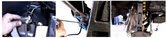
19. Tighten the new brake lines, per reversing the above steps.
