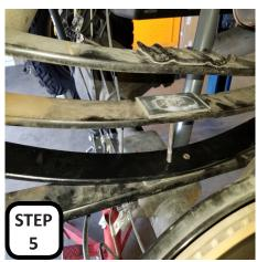
STEP 4: Loosen the clamps and separate the leaf pack.
