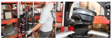
7) PLACE STRUT SPACER ON TOP OF THE STRUT AND TIGHTEN USING FACTORY HARDWARE.
