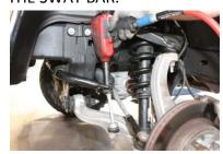
**3)** REMOVE THE LOWER STRUT BOLT THEN REMOVE ALL THREE NUTS AT THE TOP OF THE STRUT.
