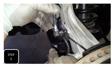
**Step 5** For newer models the whole spindle will need to come off to safely install the spacers so start by unbolting both the Brake line and ABS line from the neck of the spindle and separate.
