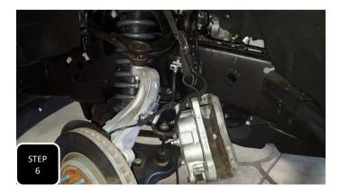
**Step 6** Unbolt the brake caliper from the spindle and support it out of the way. **NOTE: NEVER ALLOW THE CALIPER TO HANG BY THE BRAKE LINE.**
