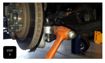
**Step 3** Unbolt the tie rod from the spindle and break it loose by hitting the side of the spindle, right at the tie rod, with a hammer. **NOTE: NEVER HIT THE TIE ROD ON THE THREADS.**
