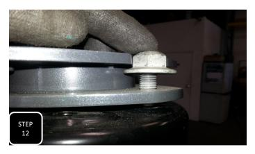
**Step 12** For 2004-2013 models, attach the strut spacer to the top of the strut with either the factory nuts or the provided nylock nuts. For 2014 and newer models, the factory nut will hit the tube on the spacer so you have to use the provided nylock nut to attach the spacer to the strut.
