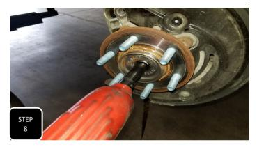
**Step 8** For 4wd models, you will need to remove the dust cap at the middle of the wheel bearing and then remove the axle retainer nut.
