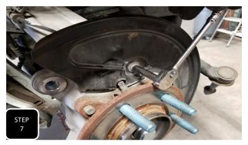
**Step 7** Unbolt the ABS sensor and position it out of the way. The top bolt of the dust shield will need to be removed for the ABS wire to clear and the sensor to be separated from the spindle.
