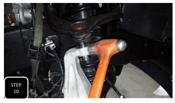
**Step 10** All models, unbolt both the upper and lower ball joints, but do not remove the nuts. Hit the side of the spindle, right at each ball joint, with a hammer to break them loose. The nuts will catch the spindle. Then remove the nuts and the spindle.
