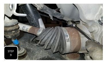
Step 9 For 4wd models, you will also need to remove the 3 hub actuator bolts on the back side of the spindle.
