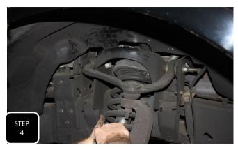
**Step 4** For 2004-2013 trucks, unbolt the 3 nuts at the top of the strut and the one bolt at the bottom of the strut then remove the strut. **Skip to step 12 for strut spacer install.**
