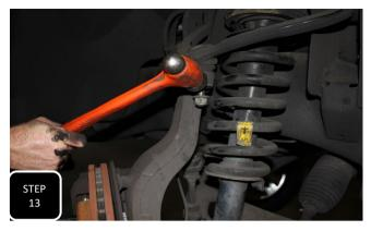
**Step 13** For 2004-2013 models you can loosely attach the top of the stut to the frame, then you will need to loosen the upper ball joint nut and then brake the ball joint loose by hitting the side of the spindle with a hammer. **NOTE: NEVER HIT THE BALL JOINT ON THE THREADS.**
