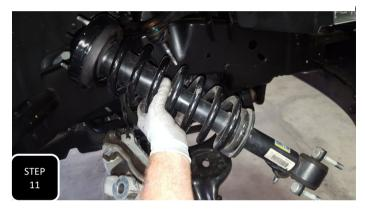
**Step 11** Push down on the lower control arm with your knee or a pry bar while also lifting up on the upper control arm so that the studs on the top of the strut clear the tower and you can remove the strut.
