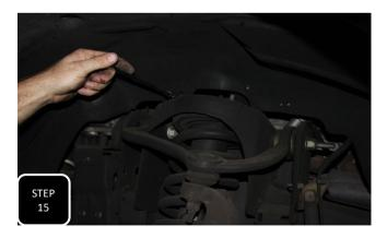
**Step 15** Re-attach the tie rod and tighten. Then tighten the 3 nuts at the top of the strut. **NOTE: DO NOT TIGHTEN THE LOWER STRUT BOLT UNTIL THE TRUCK IS ONN THE GROUND AT RIDE HEIGHT.**
