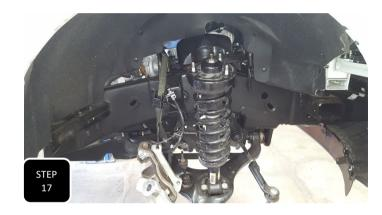
**Step 17** Push down on the lower control arm with your knee or a pry bar while also lifting up on the upper control arm so that the studs on the top of the strut clear the tower. **NOTE: THIS WILL BE TOUGHER THAN THE REMOVAL BECAUSE THE STRUT IS NOW LONGER.**
