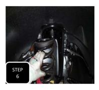
**Step 6** Lower the axle down and remove the coil with the rubber isolator.
