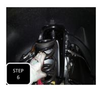
**Step 6** Lower the axle down enough to make room for the new spacer.
