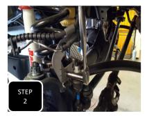
**Step 2** Un-bolt the brake line bracket from under the coil seat on both sides and separate.
