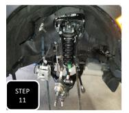
**Step 11** Place the strut assembly into the lower control arm and pry down on the lower control arm using a big pry bar while pushing the strut into the coil bucket.
