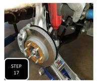
**Step 17** You will once again need to compress the coil to attach the tie rod to the spindle. Once compressed, tighten using the factory nut.
