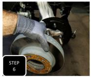
**Step 6** Remove the brake rotor and place it safely out of the way.
