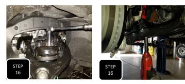
**Step 16** Tighten down the top and bottom strut studs using the provided flange nuts at the top and the factory flange nuts at the bottom.
