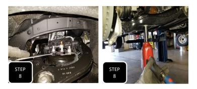
**Step 8** Remove the nuts at the top and bottom of the strut and remove the strut. You will need to push down on the lower control arm with a prybar or your knee to get the strut assembly out.
