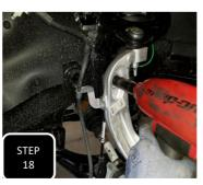
**Step 18** After the spacers have been installed on both sides of the truck, then you can attach the sway bar end links to the spindle and tighten.
