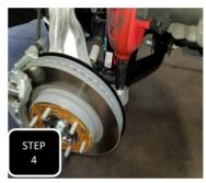
**Step 4** Unbolt the tie rod from the spindle and separate. If the tie rod does not pop out by itself, hit the side of the steering arm with a hammer right where the rod end goes through it.
