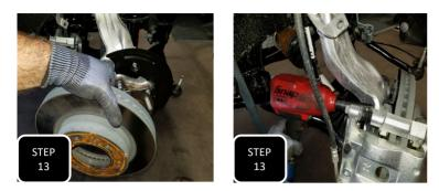
**Step 13** Install the braek rotor and then the brake caliper and tighten down both of the caliper mounting bolts.
