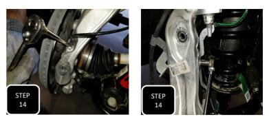
**Step 14** Install the ABS sensor and re-attach the two guides at the neck of the spindle and the control arm.
