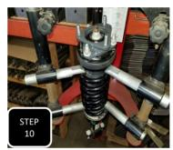
**Step 10** Because the bolt pattern is being rotated to clear the factory studs, the strut assembly will need to be placed in a strut compressor so that your can rotate
