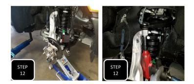
**Step 12** Jack up the lower control arm to compress the coil so that you can now re-install the spindle. Attach the spindle to the upper and lower control arms using the factory nuts and tighten.
