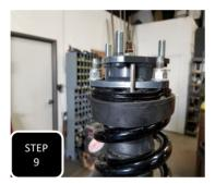
**Step 9** Install the new strut spacer and tighten using the factory flange nuts.
