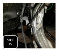
**Step 15** Re-attach the brake line guide to the neck of the spindle using the factory bolt and tighten
