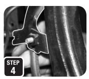
**STEP 4:** Next, remove the clip at the upper ball joint nut, loosen the nut but do not remove, and break the ball joint loose by hitting the side of the spindle with a hammer. The nut will catch the spindle, then remove the nut *(never hit the ball joint on the threads)*.
