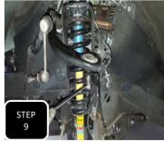
**Step 9** Place a floor jack under the lower control arm and jack up to compress the coil. Now re-attach the upper control arm to the spindle, tighten the castle nut, and reinstall the factory clip.
