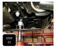
**Step 21** Re-install the skid plate using the provided 3/4" tall spacers along with the provided M8-1.25 x 40 bolts and washers near the diff and the facory bolts near the front bumper.
