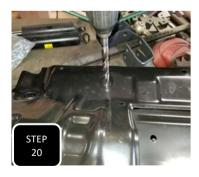
**Step 20** Once the diff drop spacers are tight, locate your primary skid plate. Using a 1/2" drill bit, enlarge the two forward most mounting holes.
