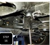
**Step 16** If your truck is equipped with a secondary skit plate directly below the differential, then remove the front two mounting bolts and for:
