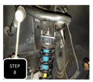
**Step 8** Re-install the strut assembly back into the truck and loosely attach the hardware at the top and bottom.
