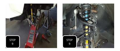
**Step 9** Place a floor jack under the lower control arm and jack up to compress the coil. Now re-attach the upper control arm to the spindle, tighten the castle nut, and re-install the factory clip.
