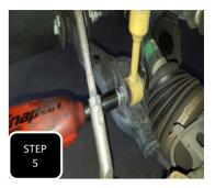
**Step 4** Unbolt the sway bar end link from the neck of the spindle and separate.
