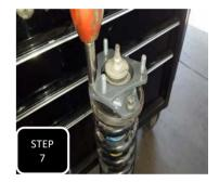
**Step 7** Remove the strut and then attach the strut spacer to the top of the strut using the factory nuts and tighten.
