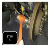
**Step 3** Loosen the tie rod nut, then break the tie rod loose by hitting the side of the steering arm with a hammer and separate. **NOTE: NEVER HIT THE TIE ROD ON THE THREADS.**
