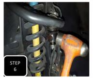
**Step 6** Remove the clip at the upper ball joint and then loosen the nut, but do not remove. Break the ball joint loose by hitting the side of the spindle with a hammer, the nut will catch the spindle, then separate. **NOTE: NEVER HIT THE BALL JOINT ON THE THREADS.**
