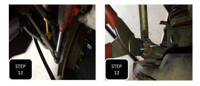
**Step 12** Re-attach the tie rod to the spindle and tighten. Once tight, re-install the factory cotter pin.
