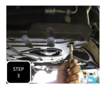
**Step 3** Raise the vehicle up and remove the skid plate by unbolting all 4 mounting bolts.
