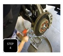
**Step 4** Unbolt the nut attaching the tie rod to the spindle and break it loose by hitting the side of the spindle with a hammer. **NOTE: NEVER HIT THE TIE ROD ON THE THREADS.**
