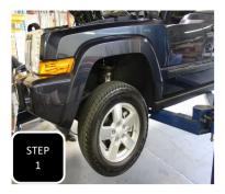
**Step 1** Jack up the front of the vehicle and support under the frame with jack stands.
