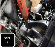
**Step 2** Open the hood and unbolt the fuse box mounting panel and the coolant tank to gain access to the strut tops then unbolt all 8 strut top bolts.
