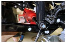
5. Remove Coil Springs and isolator.
