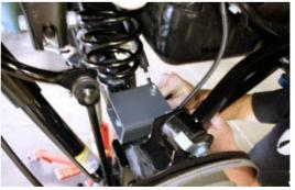
21. Install new upper shock extenders w/ new supplied hardware.
