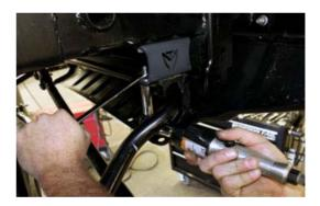
12. Install Max Trac brake line extender brackets to frame, using original hardware at the frame, and new hardware for the lower mounting holes.
