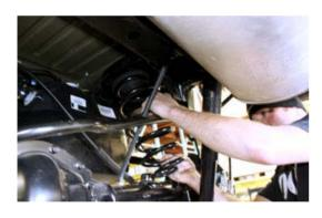
18. Set welded nut plate in through top of the frame in coil bucket. Install rear spacer w/the new 1/2" bolt and lock washer. Install spring isolator.
