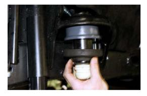
9. Install coil springs, with bump stop spacer loose. After spring is in place, tighten bump stop spacer with self tapping bolt.
