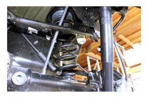
20. Install bump stop spacer to axle housing with new hardware, angle towards front.
