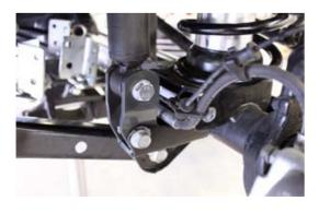
8. Locate bump stop spacer, center it on the front axle bump stop plate. Center punch, drill 11/32" hole & tap with self tapping bolt supplied in kit. Remove spacer & set in coil spring for installation.
