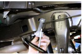
23. Install new emergency brake cable guide drop down bracket.
