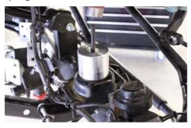
10. Install Max Trac sway bar drop down bracket using original hardware for frame.
