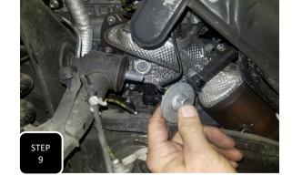
**Step 9** Unbolt the upper control arm and remove the nut.
