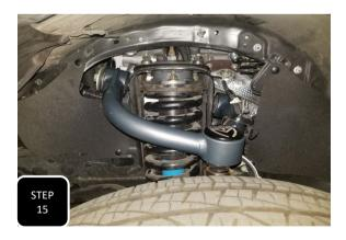
**Step 15** Lower the truck back to ride height, move the truck forward and back a few feet to settle the suspension, and then tighten the upper control arm mounting bolt and torque to factory specs.
