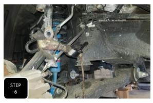
**Step 6** Once separated, use a strap to keep the spindle close to the frame. This will help prevent the brake line and ABS line from getting over stretched.
