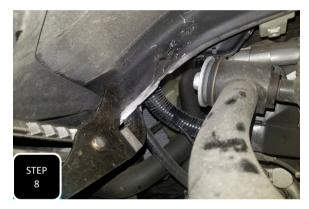
**Step 8** Using a large pair of pliars, bend the lip of the fender well outward to make room for the upper control arm mounting bolt to push out and past it. **NOTE: BE CAUTIOUS TO NOT PINCH OR DAMAGE ANY WIRING WHILE PERFORMING THIS STEP.**
