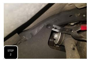
**Step 2** Gently pry to remove all of the clips attaching the rubber skirts on both sides of the control arm and remove the rubber skirts.
