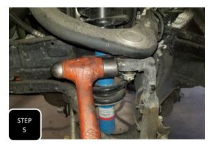
**Step 5** Loosen the nut attaching the upper ball joint to the spindle then hit the side of the spindle, right at the ball joint, with a hammer to break it loose. The nut will catch the spindle, then remove the nut. **NOTE: NEVER HIT THE BALL JOINT DIRECTLY ON THE THREADS.**
