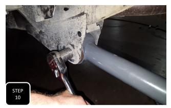
**Step 10** Locate your new lower control arms and pre-adjust the length of them according to the chart at the bottom of this page. **NOTE: DO NIGHT FULLY TIGHTEN UNTIL ALL 4 CONTROL ARMS HAVE BEEN INSTALLED.**
