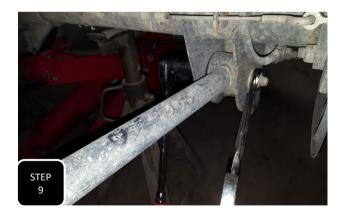
**Step 9** Loosen and remove both lower control arm mounting bolts and then remove the lower control arm.
