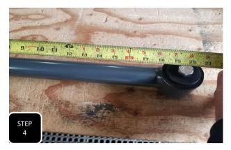
**Step 4** Adjust the new arms according to the chart on the last page of the instructions. Control arm lengths will vary based on lift height and if castor correction brackets have been installed.
