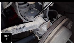
**Step 8** Working on one side at a time, loosen the upper control arm at both ends and remove the arm. **NOTE: IF YOUR JEEP IS LIFTED AND HAS BUMP STOP EXTENSIONS BOLTED TO THE AXLE THEN YOU WILL NEED TO REMOVE THEM IN ORDER TO REMOVE THE UCA MOUNTING BOLT.**
