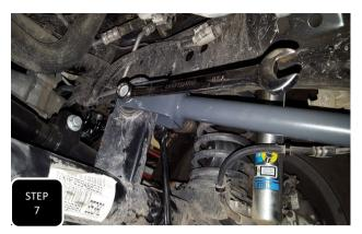
**Step 7** Repeat steps 1-6 on the other side and then fully tighten all eight control arm bolts. Lastly, re-install the factory height shields over the upper control arm mounts only if you do not have castor correction bolts.
