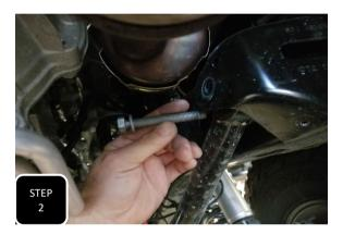
**Step 2** Working on one side at a time, remove both bolts attaching the upper control arm to the axle and the frame, then remove the control arm.
