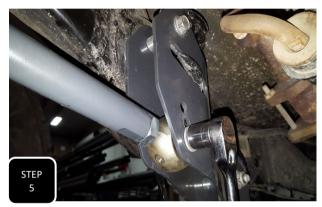
**Step 5** Loosely attach the new upper control arm using the factory bolt at the axle and the provided 7/16" bolt at the frame side. **NOTE: DO NOT FULLY TIGHTEN UNTIL ALL 4 ARMS HAVE BEEN INSTALLED.**
