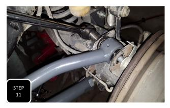
**Step 11** Pre-adjust your new upper control arm and then loosely install it. Next, repeat steps 8-11 on the other side and then fully tighten all 4 control arms.
