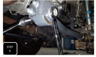
Step 6 Loosely install the lower control arm utilizing the factory bolts at both ends of the arm.
