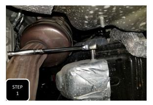
**Step 1** Unbolt the heat shields covering the upper control arm bushings at the frame, then remove and save for re-installation.
