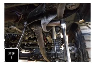
**Step 3** Remove the bolts attaching the lower control arm to the frame and the axle on the same side as the upper control arm you just removed and remove the arm.
