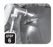
STEP 6 continued: Use the factory hardware and the provided crush tubes to loosely install the new brackets. (THE SMALLER CRUSH TUBE WILL ALIGN WITH THE UPPER MOUNT AND THE LARGER WITH THE LOWER)
