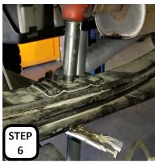
STEP 5: Install the new center pin into the over load spring and then install the add-a-leaf on top of the over load spring.
