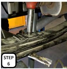
STEP 6: Allow the center pin to sit on top of the spring perch and jack up the axle until you can attach the nut and tighten.
