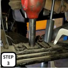
STEP 2: One side at a time, loosen and remove both U-bolts.
