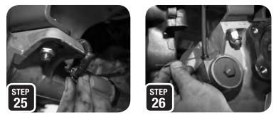
STEP 25: Plug the diff pig tail back into the diff and re-attach all
