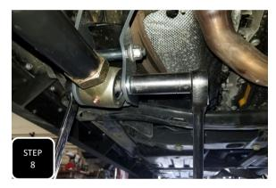
**Step 8** Tighten down both control arm bolts. The upper arm bolt should be torqued to 60 ft/lbs where as the lower control arm bolt should be torqued to 160 ft/lbs.
