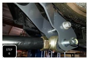
**Step 6** Loosely attach the upper and lower control arms to the new bracket using the provided hardware. The upper arm will go in the top hole if you have a 2.5" lift, the middle hole if you have a 3.5" lift, or the bottom hole if you have a 4.5" lift.
