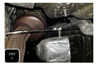
**Step 1** Unbolt the heat shields covering the upper control arm bushings at the frame, then remove and discard them.
