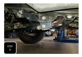
Step 9 Tighten down the 3/8" carriage bolts last and then repeat steps 1-9 on the other side.
