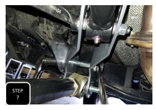
**Step 7** Once every thing is loosely installed, tighten down the bolts that attach the brackets to the frame and torque to factory specs.
