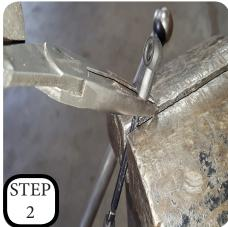
**STEP 2:** The plastic rod ends are held onto the sensor rod by a rib engaged into a retaining groove. To separate, tighten the rod into a vise and use a pair of pliers to pry the rod end off. Repeat for both rod ends.
