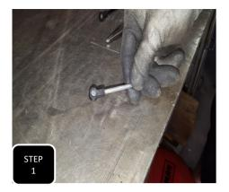
**Step 1** Separate both front sensor rods from both mounting points and remove the rods.
