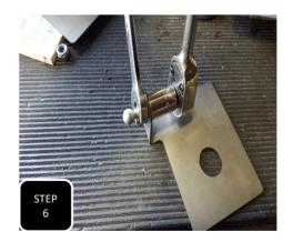
**Step 6** Attach the mounting ball to the new plate using the provided M6-1.0 nylock nut and tighten. **NOTE: REFER TO NEXT PAGE FOR AMOUNT OF DROP AND MOUNTING HOLE TO USE.**
