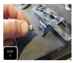
**Step 5** The rear sensor plate will need to be installed as soon as the axle is flipped and the U-bolts are ready to be installed. Loosen then remove the mounting ball from the original plate.
