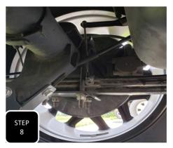
**Step 8** Once the plate is installed and the U-bolts are tight, attach the rod to the ball joint. The rear rods should clear the axle as shown. This picture shows the plate set to a 5" drop.
