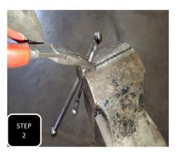
**Step 2** The plastic rod ends are held onto the rod by a rib engaged into a retaining groove. To separate, tighten the rod into a vise and use a pair of pliers to pry the rod end off. **NOTE: PLACE YOUR HAND OVER THE ROD END SO IT DOES NOT GO FLYING.**
